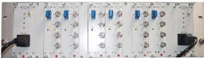
Subrack fully equipped with 2 PS, 6 FOM-400-T or 6 FOM-400-R cards
